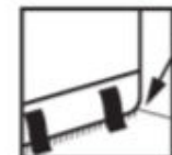
Position the Flowstop in the opening and finish inflating the top chamber.
